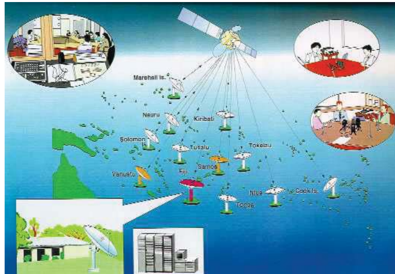
Figure 15-2: A satellite network. The “uplinks” from the ground stations to the satellite form a shared medium.
