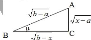
82.  $\int \sqrt{(x-a)(b-x)} dx = \frac{2x-a-b}{4} \sqrt{(x-a)(b-x)} + \frac{(b-a)^2}{4} \cdot \arcsin \sqrt{\frac{x-a}{b-x}} + C \quad (a < b)$
