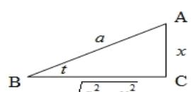
$$\begin{aligned} \therefore \int x^2 \sqrt{a^2 - x^2} dx &= \frac{a^4}{4} \cdot \frac{\sqrt{a^2 - x^2}}{a} \cdot \frac{x^3}{a^3} - \frac{a^4}{8} \cdot \frac{\sqrt{a^2 - x^2}}{a} \cdot \frac{x}{a} + \frac{a^4}{8} \cdot \arcsin \frac{x}{a} + C \\ &= \frac{x}{8} \cdot (2x^2 - a^2) \sqrt{a^2 - x^2} + \frac{a^4}{8} \cdot \arcsin \frac{x}{a} + C \end{aligned}$$
