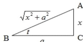
$$37. \int \frac{dx}{x \cdot \sqrt{x^2 + a^2}} = \frac{1}{a} \cdot \ln \left| \frac{\sqrt{x^2 + a^2} - a}{x} \right| + C \quad (a > 0)$$
