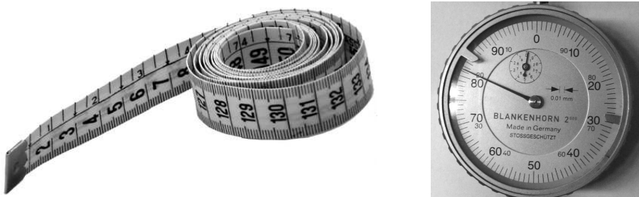
Figure 1.1: Both the tape measure and the dial are analogue devices
